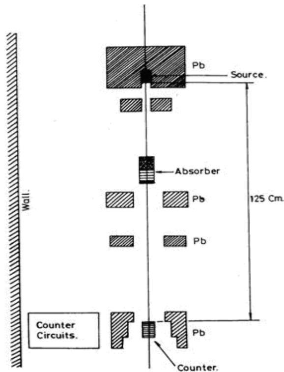
**Fig. 1 The schematic view of the experimental set up.**
