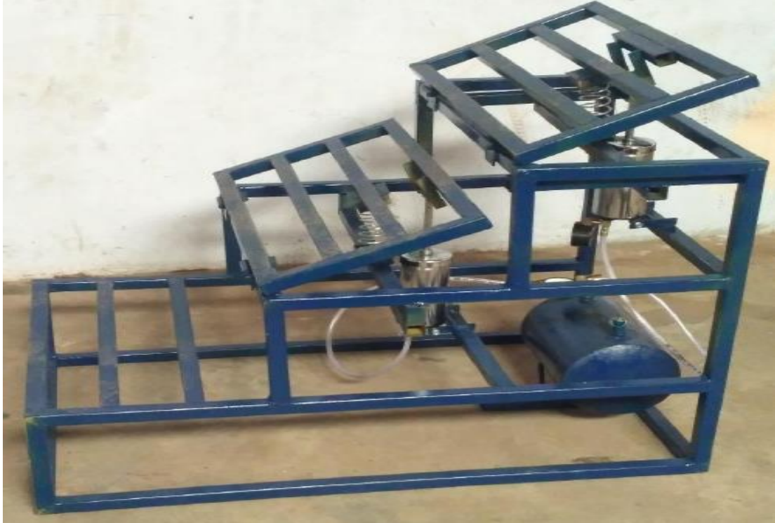
Figure 2 Photographic view of the staircase based compressed air generation setup
