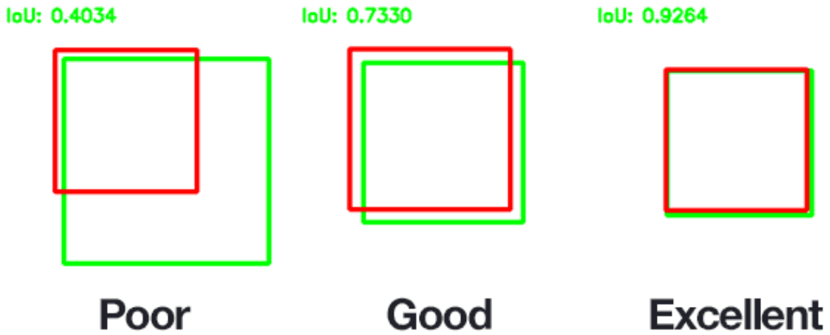
Fig. 10: Different of types of Intersection over Unions, where based on the IoU value, Poor, Good, Excellent – these three categories have been devised
