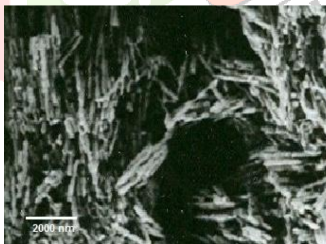
Figure 4. SEM image of CdS nanowires synthesized into AAM with pore diameter 200 nm (length of bar is 2 \mu m).
