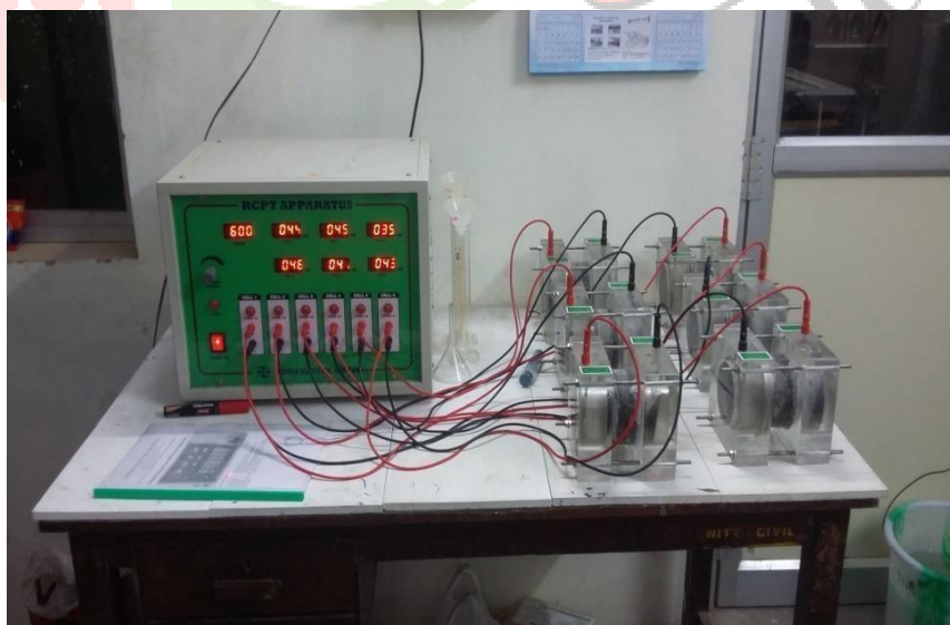
Fig. 4.2 Rapid Chloride Based Permeability Test Setup
