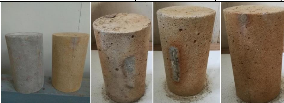
Fig. 4.3 Specimen at different cycles for 5% of dosage of acid
