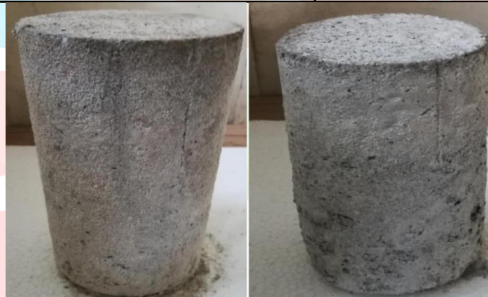
Fig. 4.4 Specimen after 4 cycles at 5% dosage of salt
