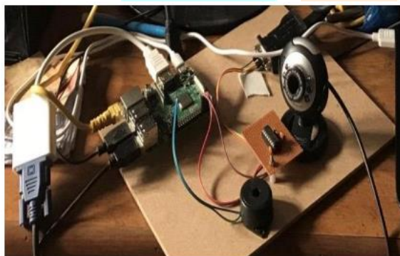
Figure 1.2: Raspberry Pi with a buzzer
