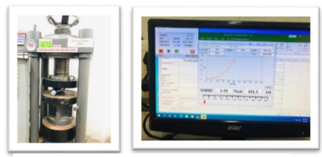
Figure 7: photograph of testing compression on plastic bottle
