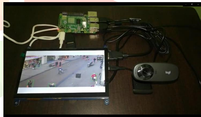
Figure 10: Social Distancing monitoring implemented on Raspberry Pi
