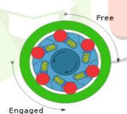
In mechanical or automotive engineering, a flywheel or overrunning clutch is a device in a transmission that disengages the driveshaft from the driven shaft when the driven shaft rotates faster than the driveshaft. An overdrive is sometimes mistakenly called a flywheel, but is otherwise unrelated.
