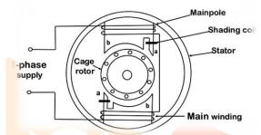
A single phase induction motor consists of a single phase winding on the stator and a cage winding on the rotor. When a 1 phase supply is connected to the stator winding, a pulsating magnetic field is produced.
