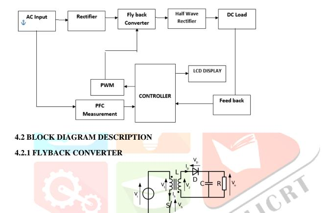
The **flyback converter** is used in both AC/DC and DC/DC conversion with galvanic between the input and any outputs. The flyback converter is a buck-boost converter with the inductor split to form a transformer, so that the voltage ratios are multiplied with an additional advantage of isolation. When driving for example a plasma lamp or a voltage multiplier the rectifying diode of the boost converter is left out and the device is called a flyback transformer.
