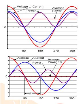
AC power flow has the three components: real power (P), measured in watts (W); apparent power (S), measured in volt-amperes (VA); and reactive power (Q), measured in reactive volt-amperes (VAr).
