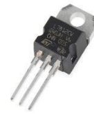
Fig: Regulator LM7812 IC diagram
