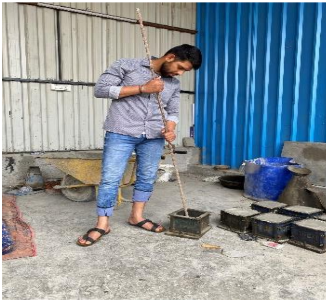
Fig.4 Material compaction by using tamping rod
