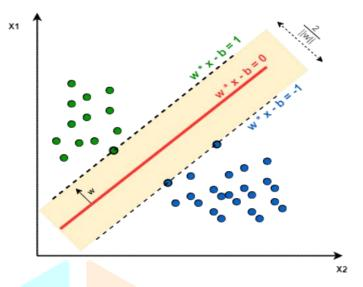
The computations of data points separation depend on a kernel function. There are different kernel functions: Linear, Polynomial, Gaussian, Radial Basis Function (RBF), and Sigmoid. Simply put, these functions determine the smoothness and efficiency of class separation, and playing around with their hyperparameters may lead to overfitting or underfitting.
