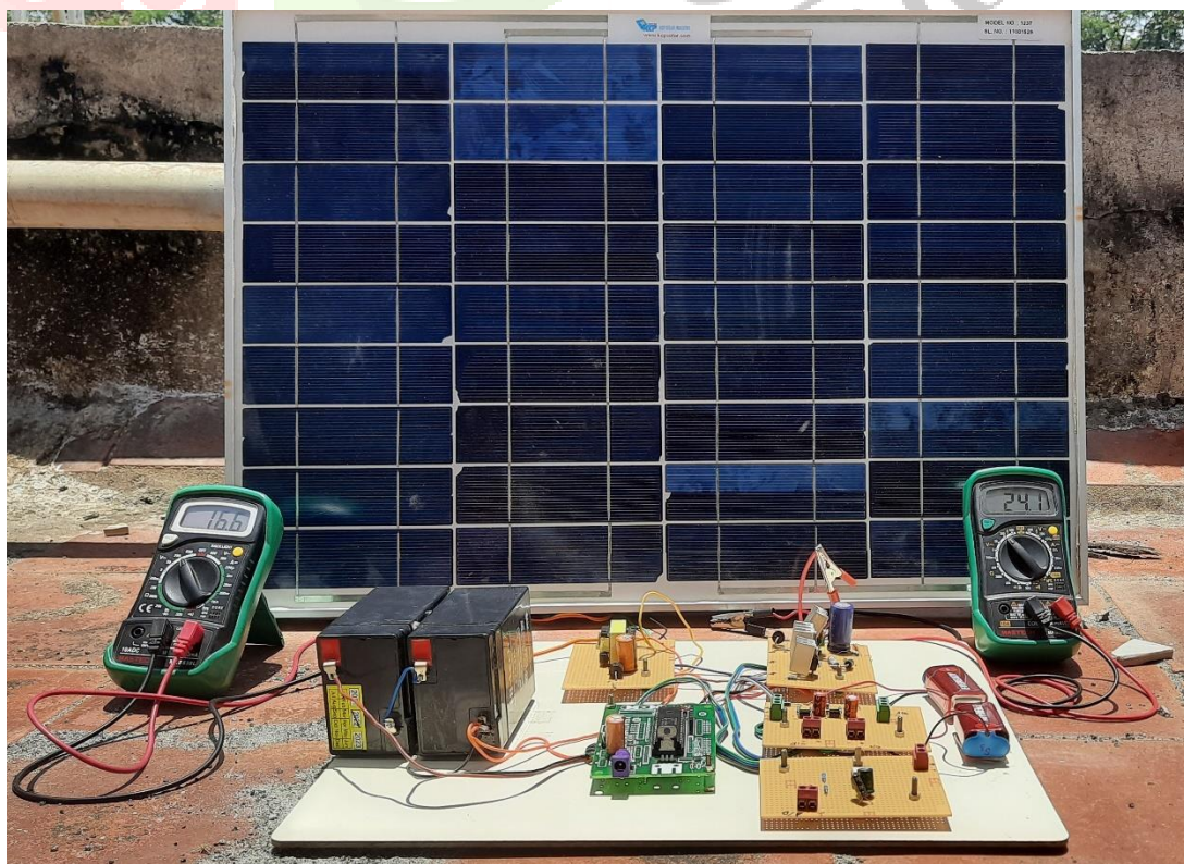
Fig.8: Hardware setup for single stage inductor based dual I/O DC-DC boost converter (DOBM)
