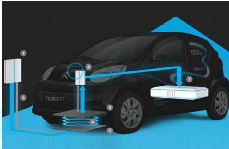
IPT-based wireless charging of an electric car.
