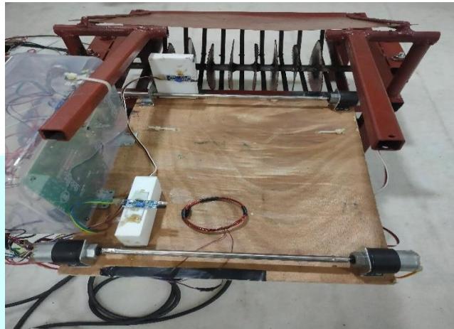
Fig 5.5. Conveyor belt assembly with 30 rpm DC motor and metal sensor
