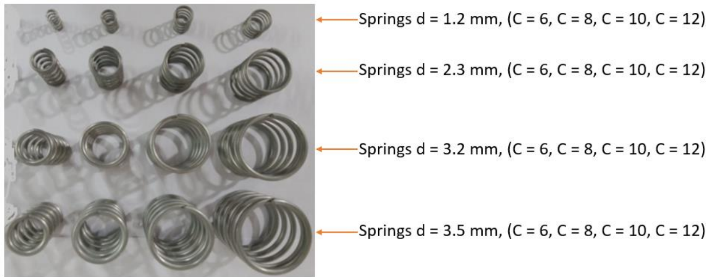
Figure 1. Sample spring made of Stainless-steel wire (1 to 16)
