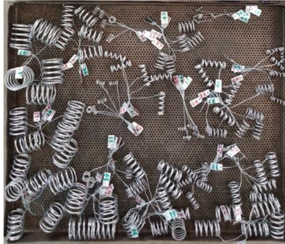
Figure 2. Stainless steel springs ready for stress relieving
