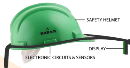
Fig 15: electronics assembled inside work helmet
