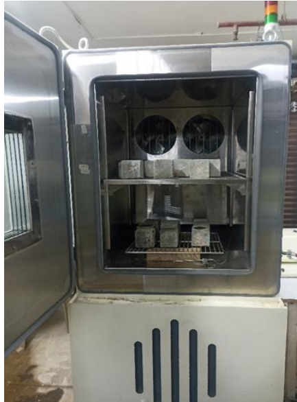
Fig. 3. Freezing-thawing of concrete specimens in freezer
