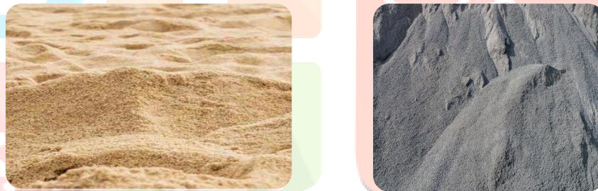
Fig:-02 Natural sand & Quarry dust
