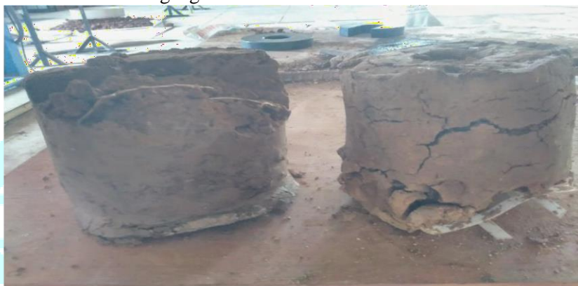
Fig-5.2 Laboratory Experiment with Geogrid in CBR Mould
