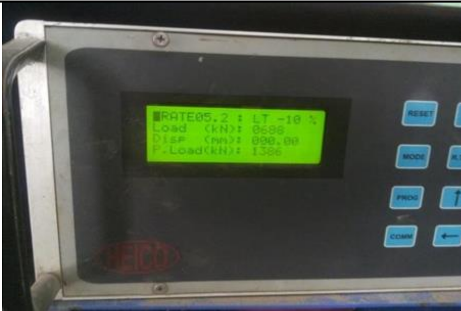
Fig. 3 Compressive load reading in KN
