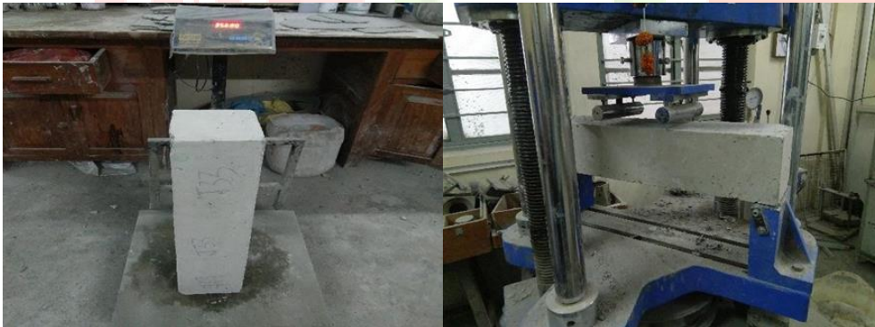
Fig. 4&5 Weight measurement and Flexural testing machine
