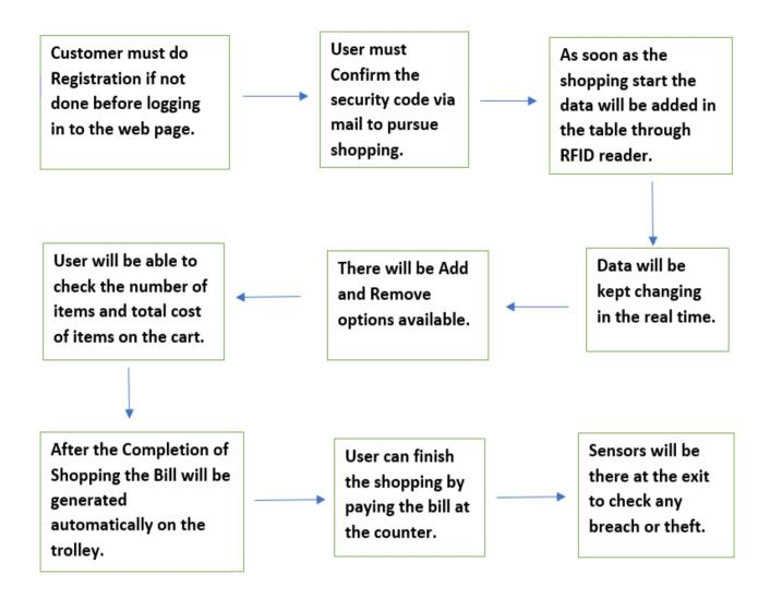
Fig: Workflow of Secure Smart Shopping Cart.
