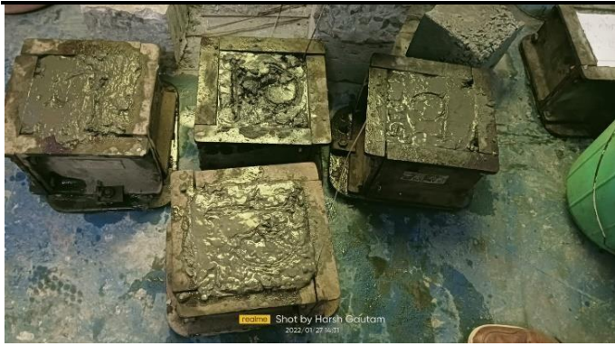
Fig.2 Casting of Sample
