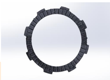
Figure. Stl. file of a clutch having little wear on its surface.
