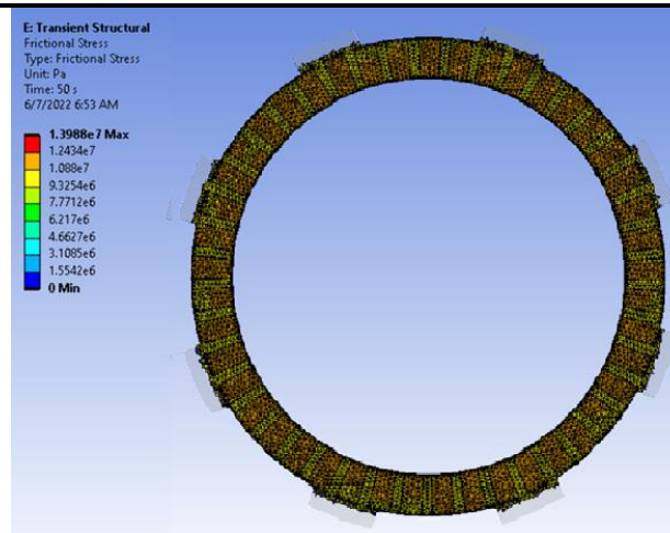
Figure. It show the Friction stress distribution on replaced clutch plate.
