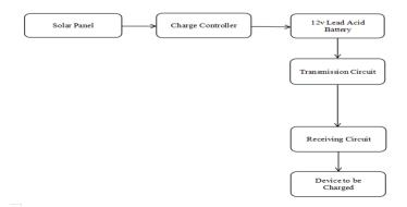
We produced and used numerous schematics and diagrams at the outset of the physical design phase. This is a crucial component of assemble since these images and texts can provide as clear directions for assembly. Our system's top-level block diagram, which displays the fundamental connectivity and power levels of each component in the system, was the first to be created. The process
