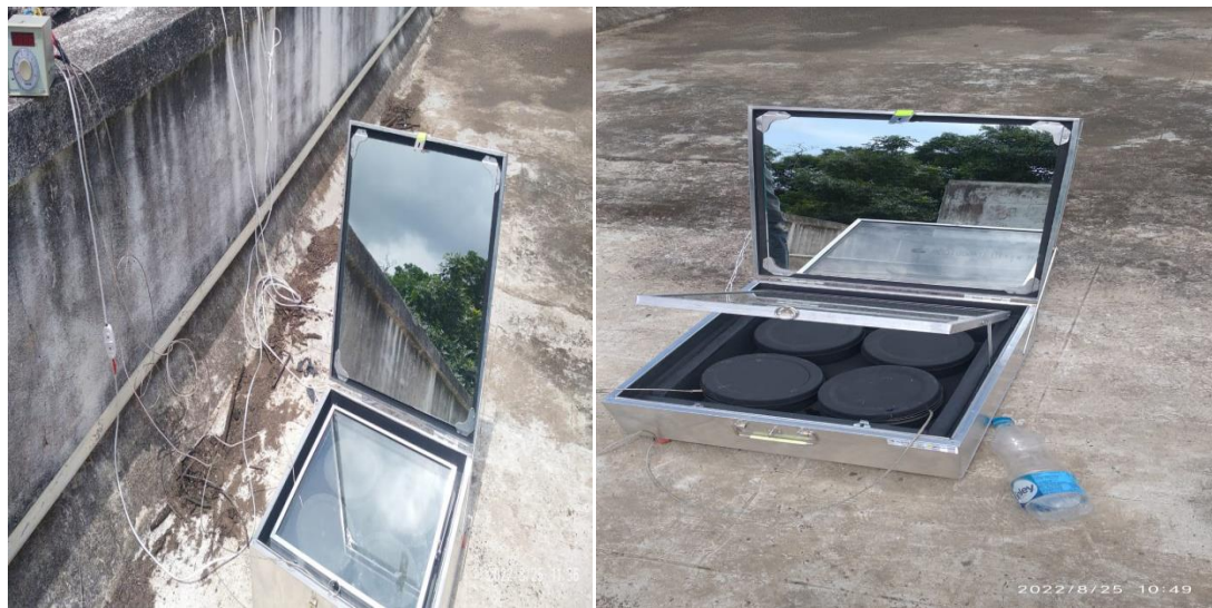
Fig.7. solar cooker before modification with cooking pot
