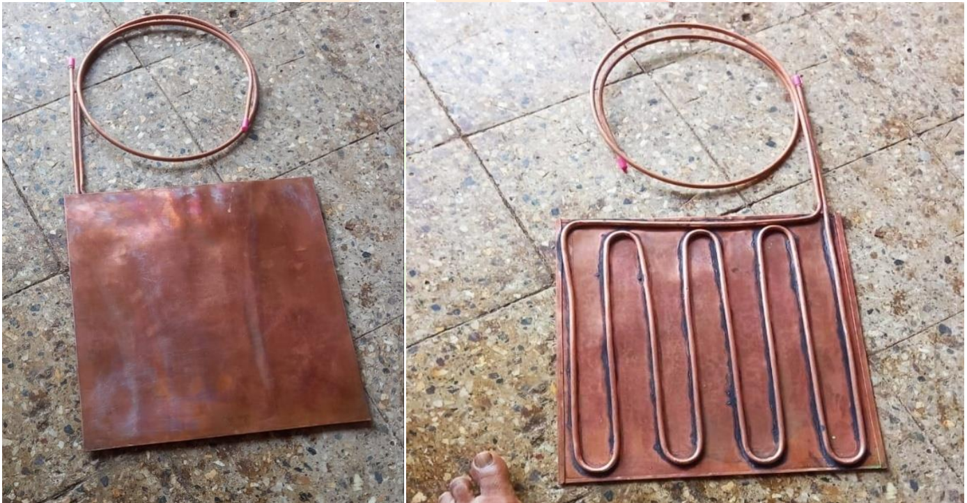
Fig.6. copper tube connected with cooper plate
