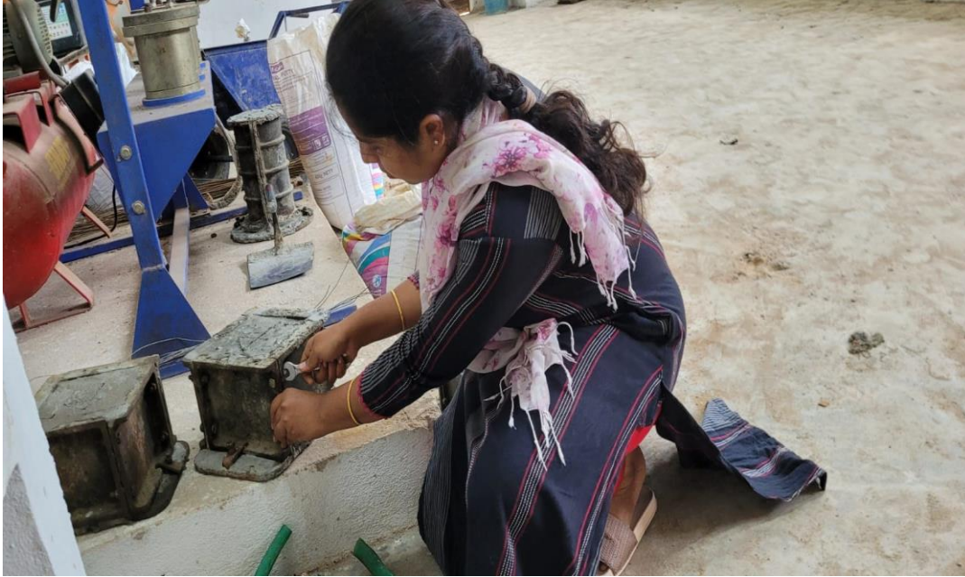
Fig 6.2 Casting of Cubes
