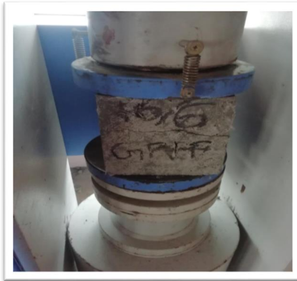
Fig 3.1: Compressive Strength Test
