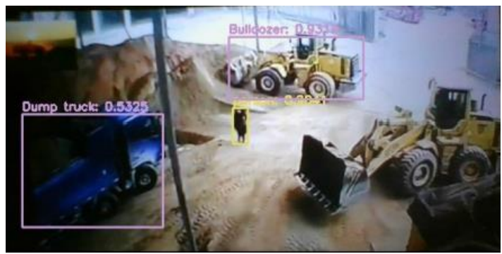
Fig 7.28: Detection of a back-over accident between a dump truck and a worker Fig 7.29: Detection of a worker in the vicinity of a dump truck and a bulldozer
