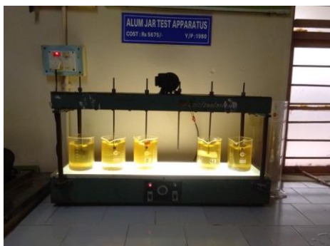
Fig 3: Chemical Coagulation Setup
