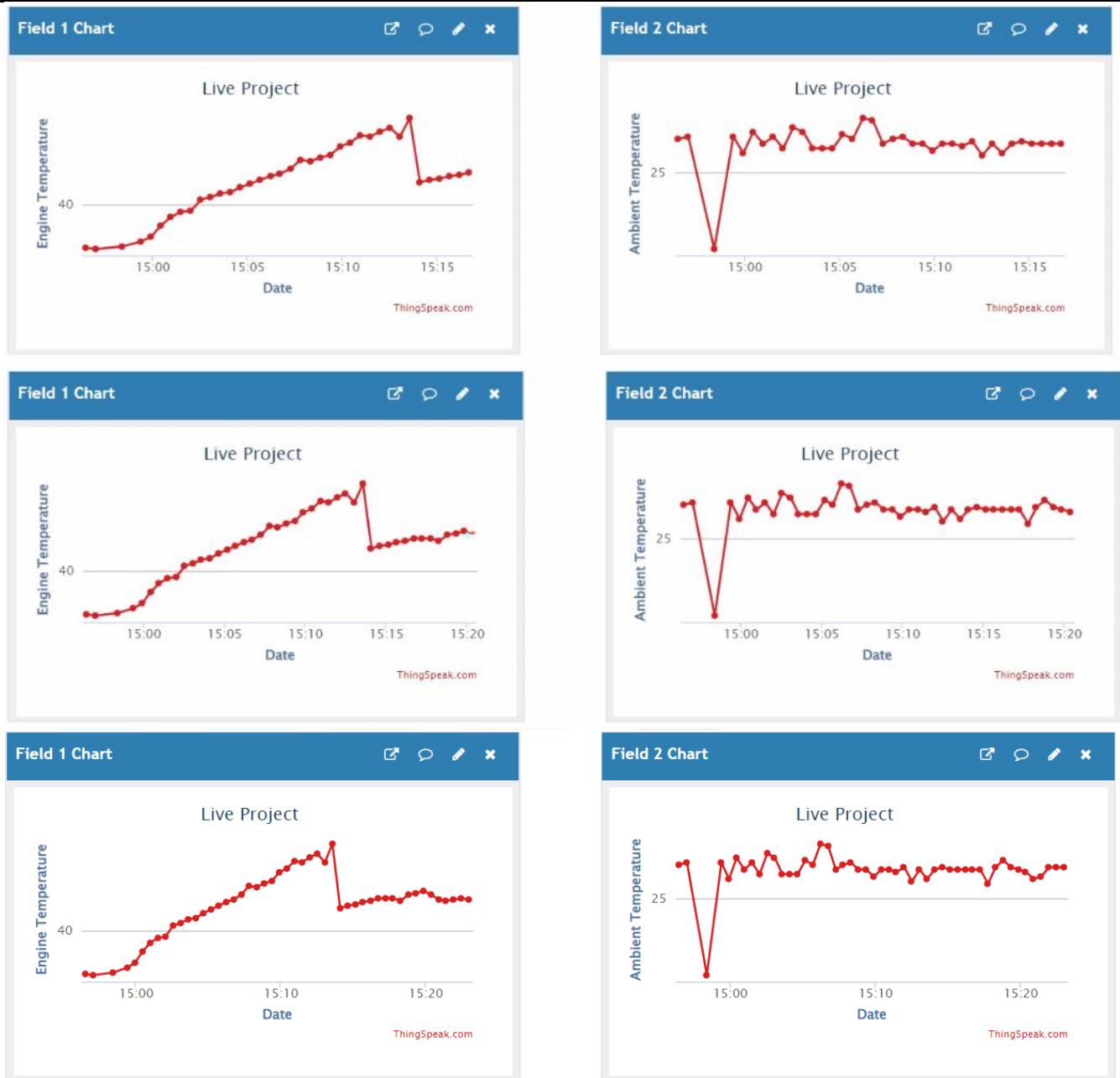
Fig 13: Values of Engine temperature Illustrated in IoT platform during the driving cycle
