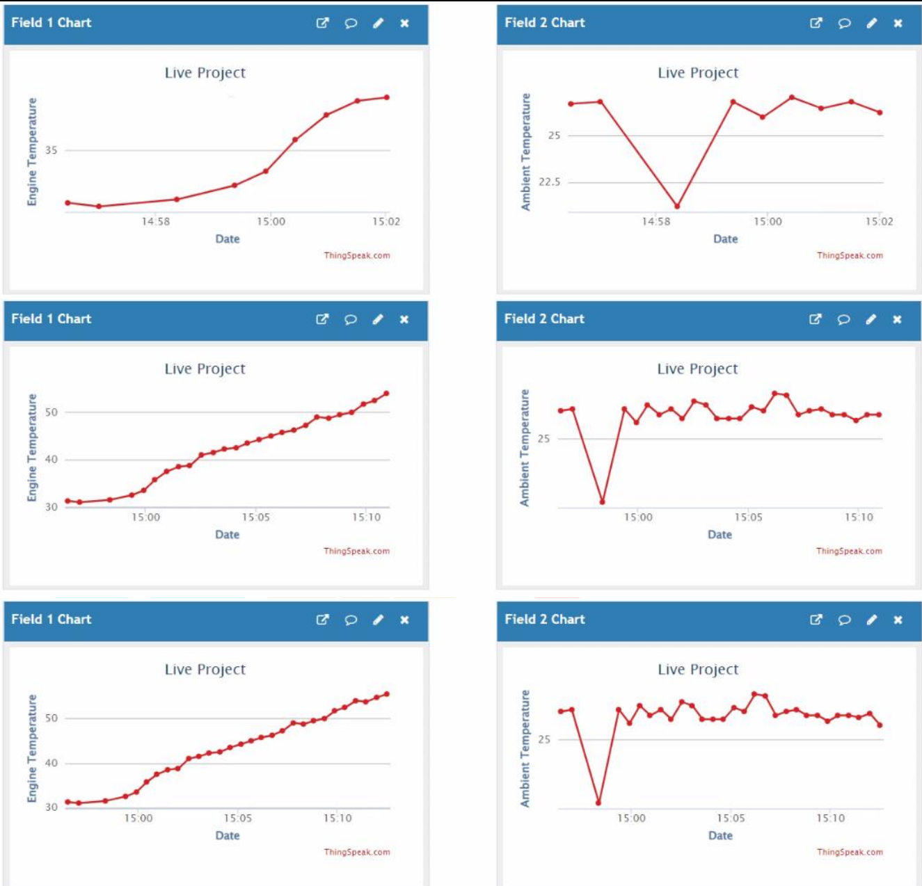
Fig 12: Values of Engine temperature illustrated in IoT platform during the idling cycle
