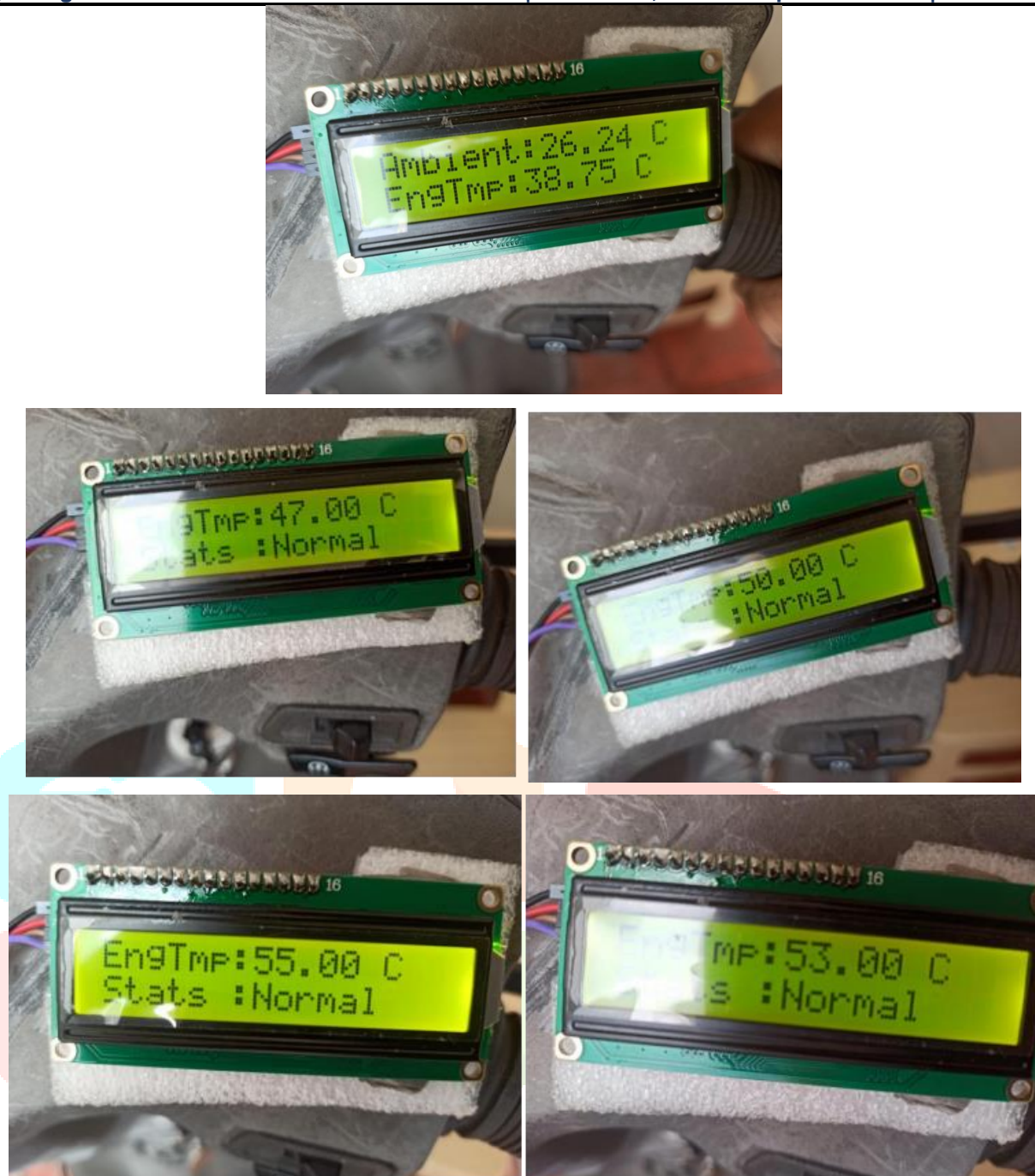
Fig 11: Values of Engine temperature displayed in LCD during the idling cycle
