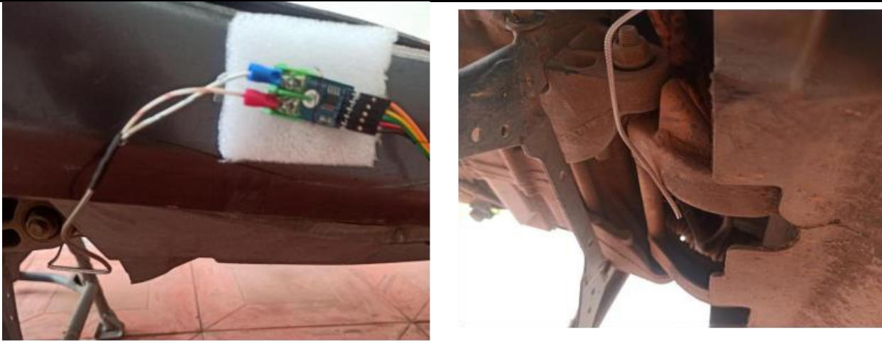
Fig 8: Attachment of Thermocouple and MAX6675 module
