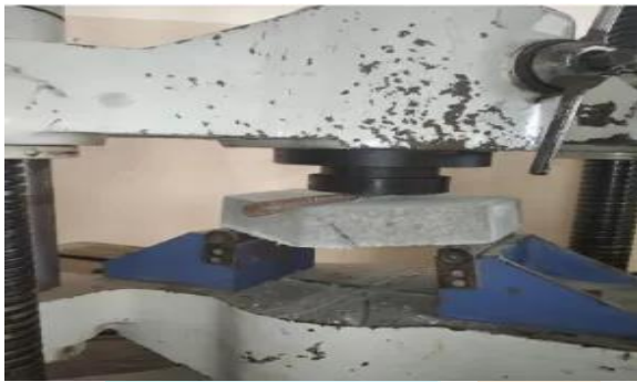
Figure 3: Flexural strength test setup
