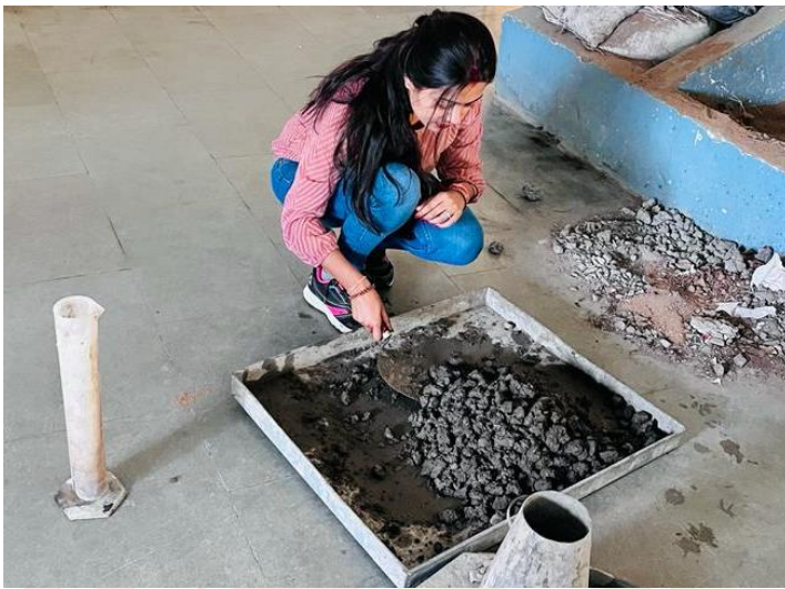
Figure 5. Casting specimen for test on hardened concrete.
