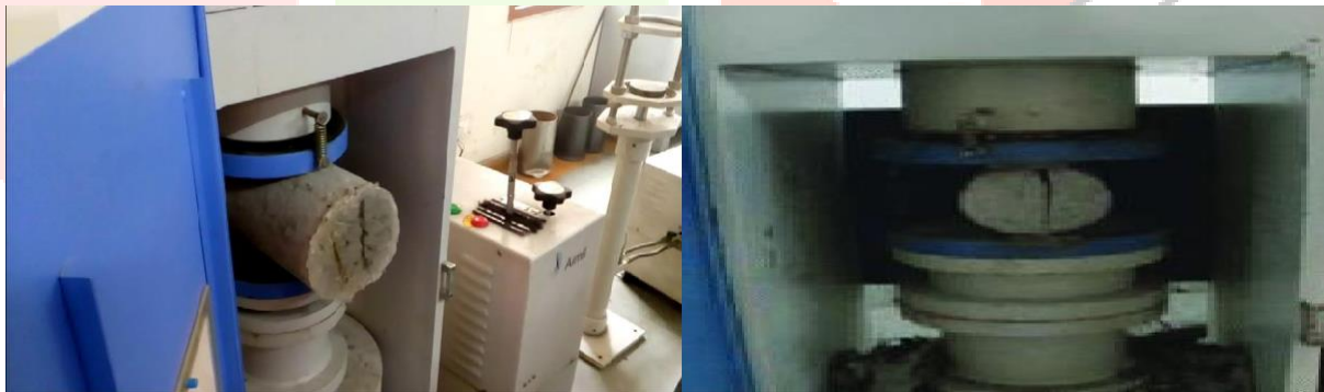
Figure 1. Split Tensile Strength Test
