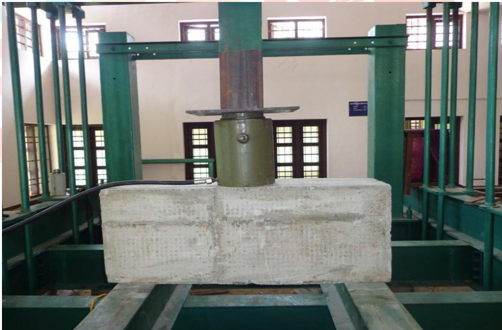
Figure 6. Test setup for infill beams & normal RCC Beam
