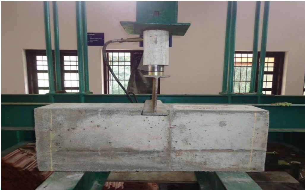
Figure 5. Test setup for Ferrocement Hollow beam
