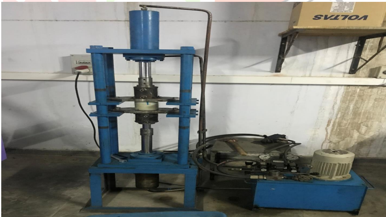
Figure 2: Assembly of AFM Set Up
