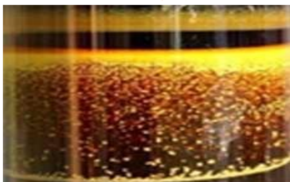
Figure 1.1 spherulite crystals are grown in gel
