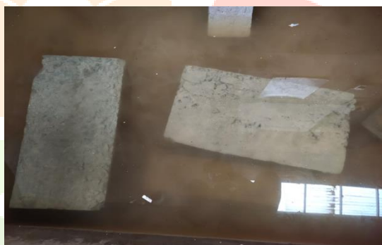
Fig. 6 Curing of column
