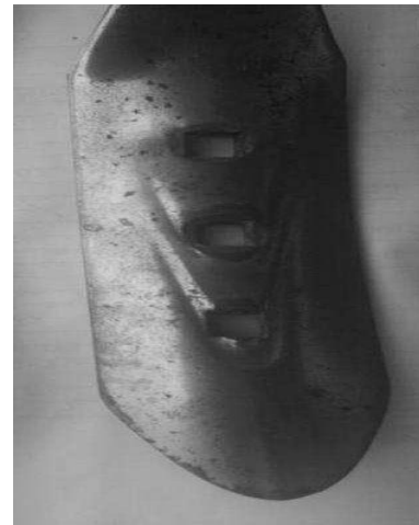
Figure.2 Worn out Reversible Shovel
