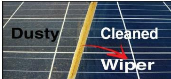
Fig.1.5 Showing half side clean and dusty panel
