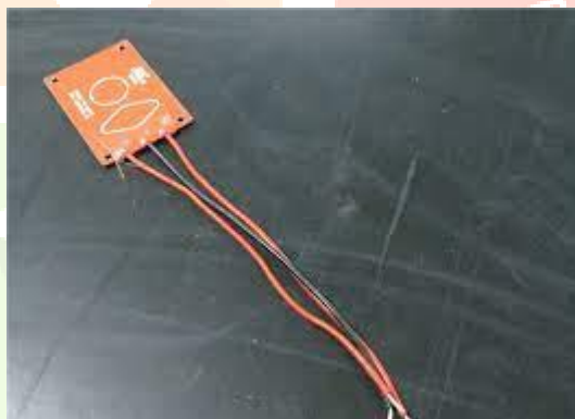
Fig:- 2.1 heating coils
