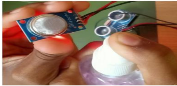
Fig:-6. Detecting Hazardous gas using an MQ2 sensor
