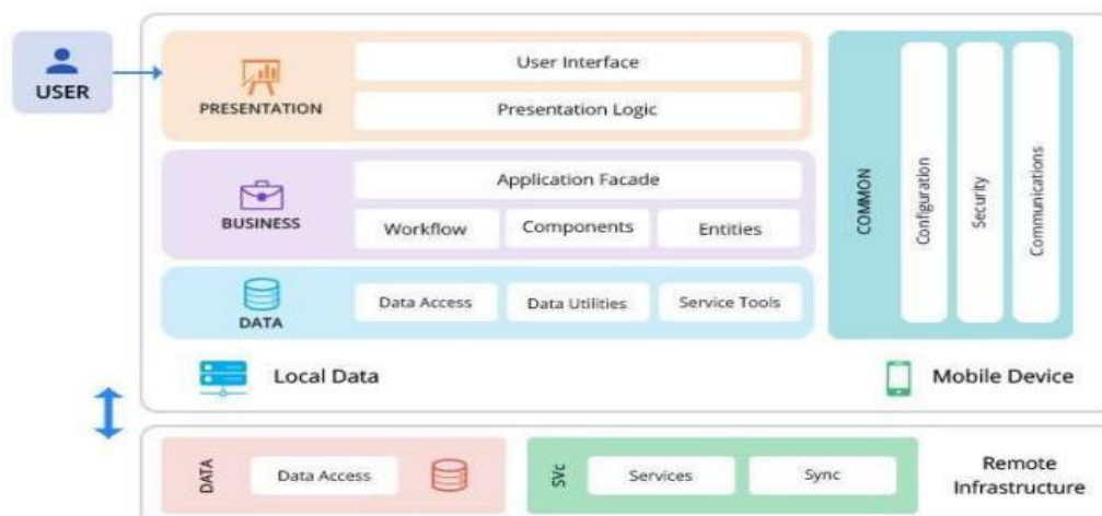
Fig. System Architecture
