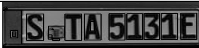
Figure 8. Contours applied in rectangular boxes form
