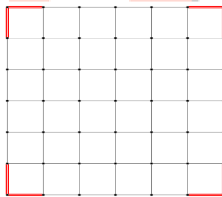
Fig 2:- Plan of Shear Wall At Position 'A'
