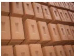
Fig-6 Compressed Rammed Earth Blocks Source UNEP-SBCI(2010)[10]
