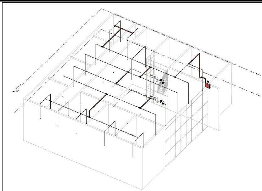
Figure.4 Typical arrangement of Fire Sprinkler system
