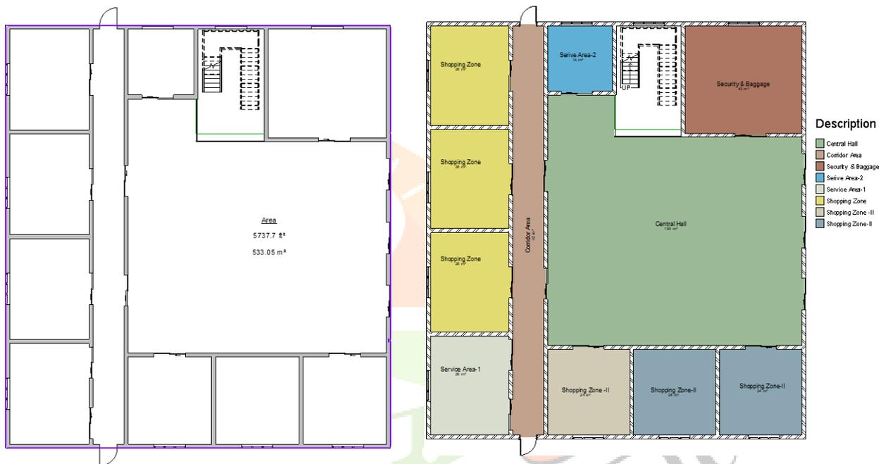
(b) Figure 1a. The Gross Floor Plan area of 514m<sup>2</sup> and 1b. Description of floor area for utilization
