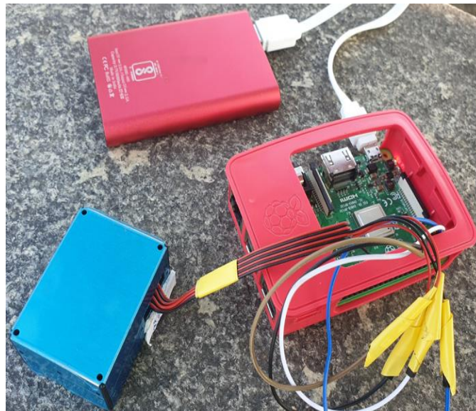
Fig1: Plant tower pms5003 sensor with Raspberry pi
