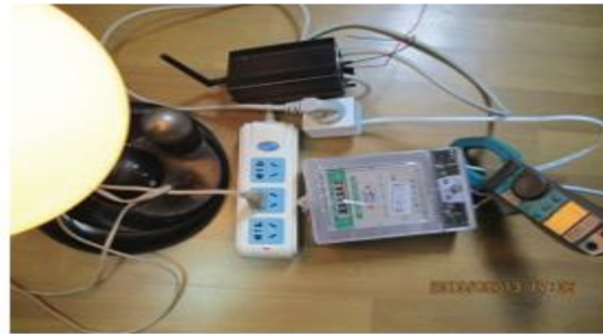
Figure 12: ZBDECS, standard wattmeter, and clampmeter.
